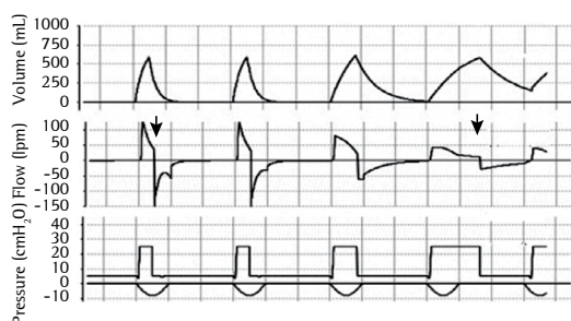
Figure 3 – Cycling asynchronies during pressure support ventilation. In the first cycle, the cutoff point of 25% of the peak inspiratory flow (percentage of the cycling criterion) was reached rapidly; the ventilator's inspiratory time was therefore shorter than the time desired by the patient. This is shown in the expiratory segment of the flow curve, which tends to return to the baseline as a result of the patient's inspiratory effort, which is still present. The last cycle represents the opposite situation, i.e., delayed cycling. The flow reduction occurs very slowly, which is typical of airway obstruction; the cycling threshold is therefore reached with some delay. Sometimes, the cycle is interrupted by a contraction of the respiratory muscles, which causes an increase above the support pressure adjusted at the end of inspiration (not shown in this figure). Figures obtained at Xlung.net, a virtual mechanical ventilation simulator. Available at: http://www.xlung.net
